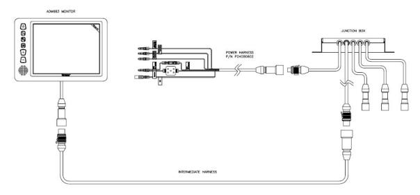
Install the **AOM713WP** monitor panel, Intermediate harness, junction box and wiring harness in place of the old system. Your camera cable will connect into the **TO CAMERA** inputs.
